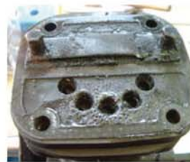
Carbon build up on valve plate
