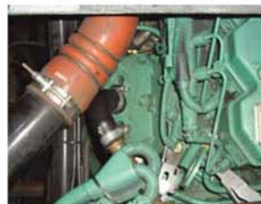
Check there is no damage or crushing of the compressor inlet pipe
